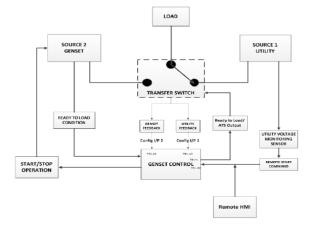
Control system - The PowerCommand® electronic control is standard equipment and provides total system integration, including auto remote start/stop, alarm and status message display.
