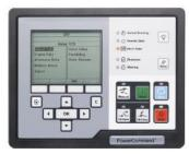
The PowerCommand control system is an integrated microprocessor based generator set control system providing voltage regulation, engine protection, alternator protection, operator interface and isochronous governing. Refer to document S-1567 and S-1570 for more detailed information on the control
