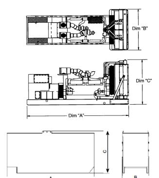
Those outlines drawings are to provide representative configuration details for model series only. See respective model data sheet for specific model outline drawing number.
